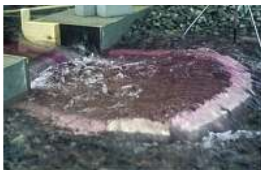
Figure 2.27: Model of the stilling basin
