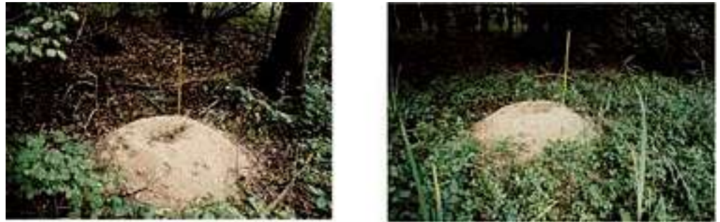
Figure 2.15: Sand craters in the hinterland of the Rhine winter dike close to Hördt, Germany
