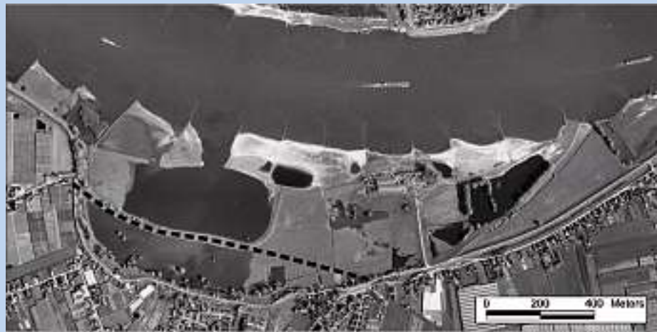
Figure 2.62: The Gamareren Floodplain along the River Waal with the new dike alignment (in 1995)
