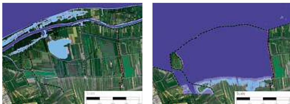
Figure 2.3: Example of a controlled retention area: Ingelheim Polder, left ecological flooded, right HQ200 flooded
